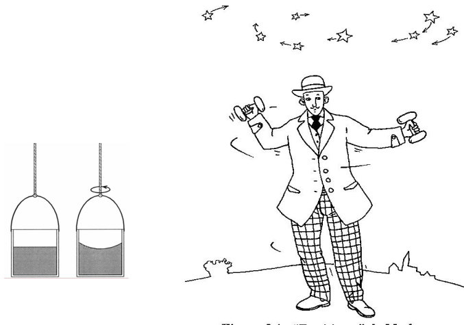
Figure: Left: Newton's rotating bucket, Right: Inertial forces caused by acceleration and simultaneous apparent rotation of distant stars.
