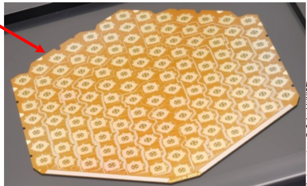
ACTPol PA1 Hex Detector Wafer (127 pixels \rightarrow most on a CMB wafer yet!)
