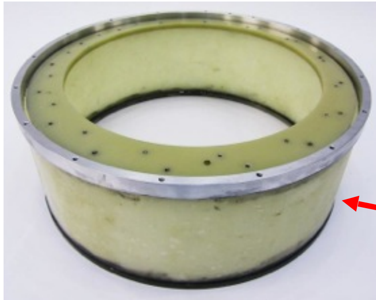
1K-0.1K Re-entrant G10 Array Suspension
