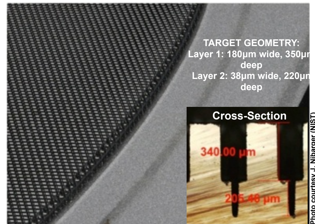
Prototype two-layer coating (on curved 150GHz lens surface)
